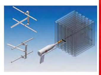
WELD-TITE MODULE Attachment is a speed weld system that requires no stud pattern or furnace layout. The advantage to this attachment system is the speed of installation. Just fire the speed weld gun which attaches the stud to the furnace casing and then tightens the module onto the stud. Nutec™ modules can be installed in a Uni-directional (with batten strips) or in a Parquet pattern.
