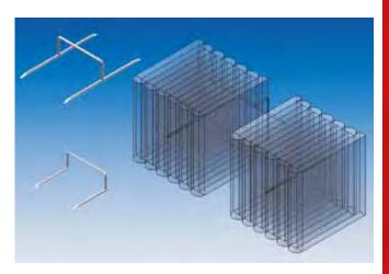
H ANCHOR MODULE Attachment can be used for standard size modules or with Macro Modules (larger size modules). This hardware system provides a strong and durable lining for longer furnace life. This attachment is quick and easy to install. The H Anchor is welded to the furnace shell and a module is slid over both sides of the anchor. Using this system, Nutec™modules can only be installed in a Uni-directional pattern with batten strips.
